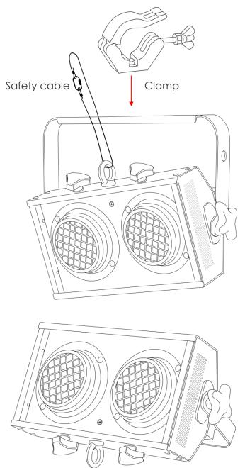
The Stage Blinder can be placed on a flat stage floor or mounted to any kind of truss with a clamp.
