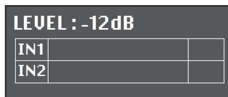
The **LEVEL** screen displays the audio levels of different inputs. This allows you to monitor the signal and adjust the input level accordingly. Once the volume is increased, the levels will be displayed as shown below:
