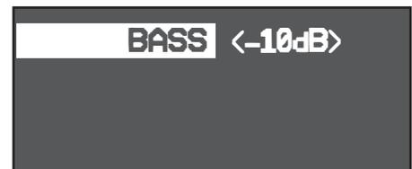
The **BASS** menu adjusts the **low-frequency** response of the speaker. The range is -10 dB to +10 dB. Select the value using the MASTER rotary knob.
