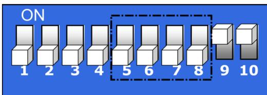
**Manual Mode:** DIP switches #9-10 to ON.
