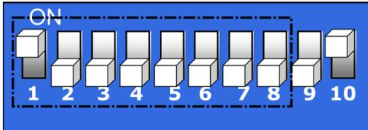
**Auto Mode:** DIP switch #9 to OFF / DIP switch # 10 to ON.
